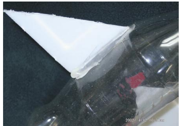
Fig. 7. Close-up of bead of hot melt glue used to attach plastic fins to plastic bottle. Put bead(s) along both sides of fins to increase ruggedness.
